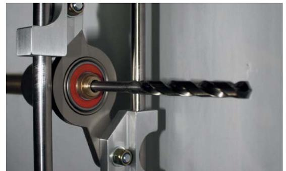
Picture showing Mortise Jig fitted with Morris MTA10 and a Morris ET101200 HSS drill bit
